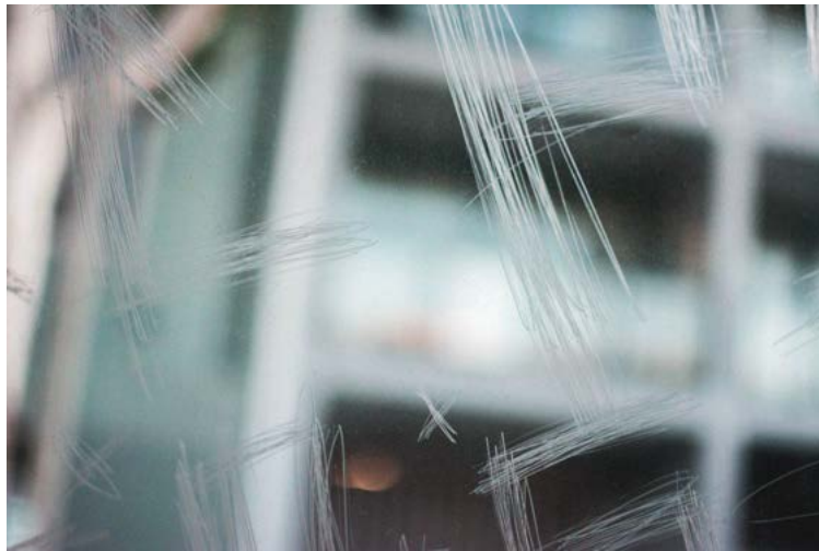
Figure 28: The use of sharp-tipped tools can scratch your build-plate surface
