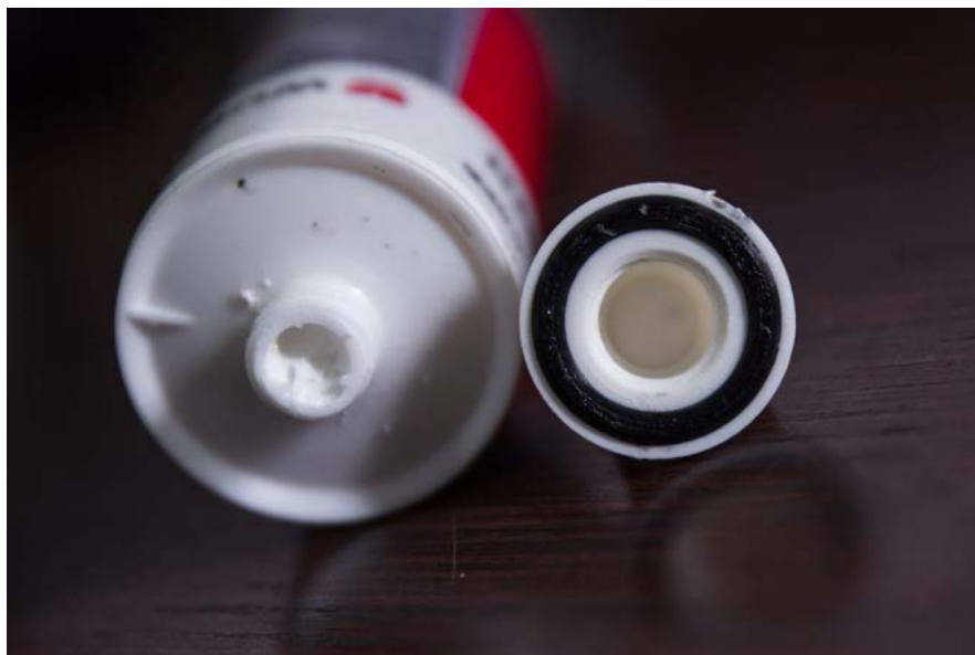
Multimaterial 3D printed cap with printed in place o-ring, The cap is made from ABS material while the O-ring is printed in DSM Arnitel 2045.
