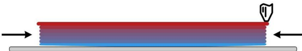
Figure 5: Print warp due to thermal gradient
