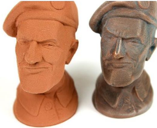
ColorFabb copperFill Metal Filament before polishing and after polishing, via: matterhackers.com
