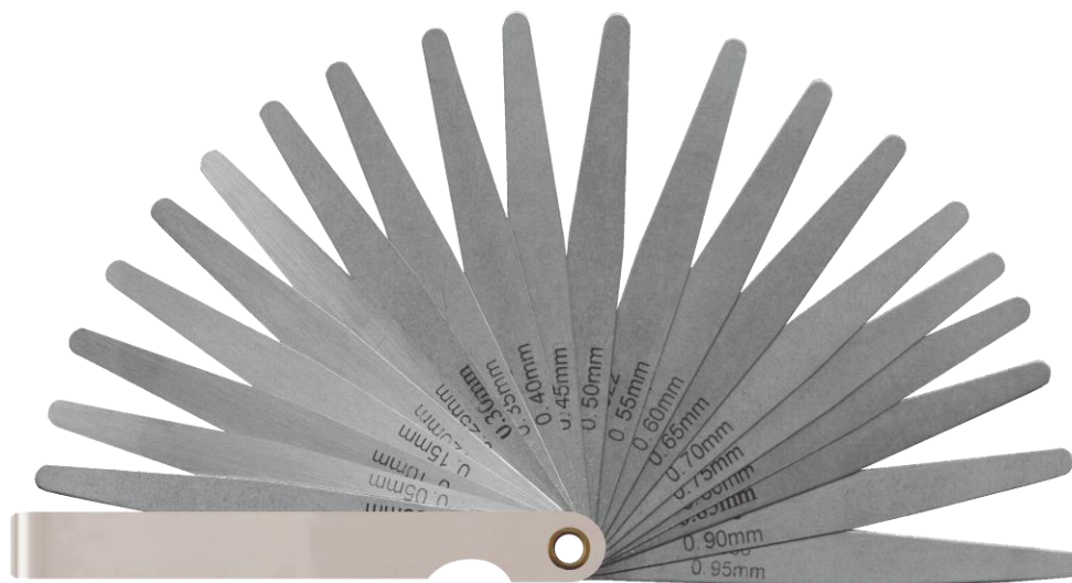
Figure 12: Feeler gauge, ideal for measuring small amounts of warp accurately
