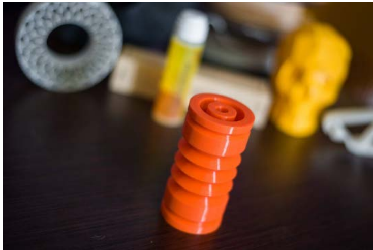
3D printed Circular Flexbellow prototype. Printed in NinjaFlex NinjaTek on a Raise3D N2 with a bondtech extruder upgrade which facilitates FDM printing of softer materials.
