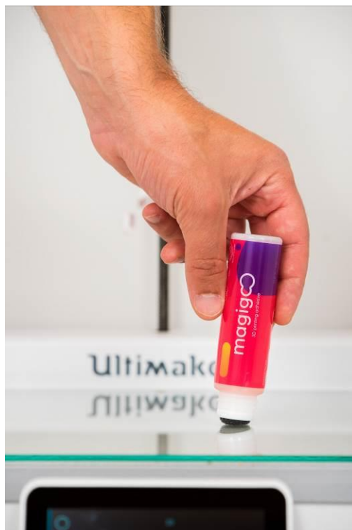
Figure 16: Apply Magigoo in an even layer on the area for printing
